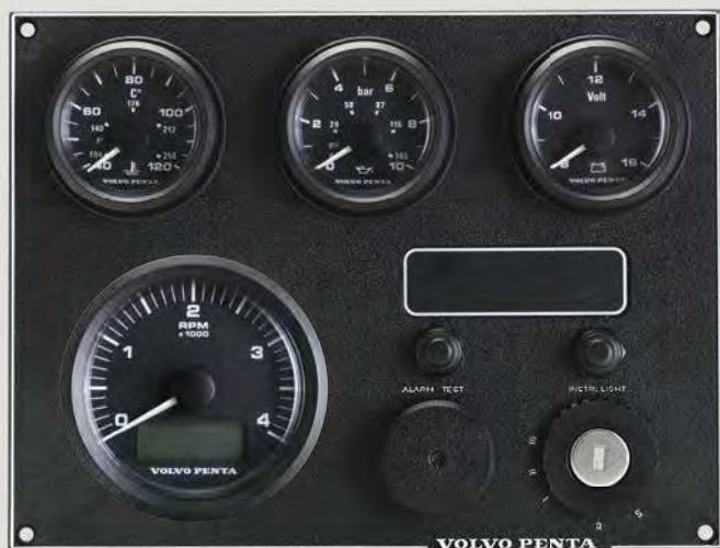
Main station panel with the tachometer (option).
