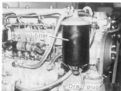
**⚠ Important:** For the separate-type fuel oil filters, remove impurities and change the element by using the procedure in Sec. 8-1-3).
